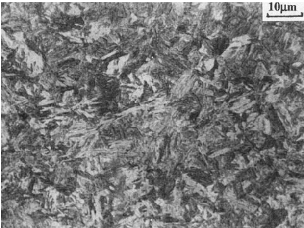
Fig. 8 Microstructure of weld metal of steel in as-quenched condition, 960 \times
